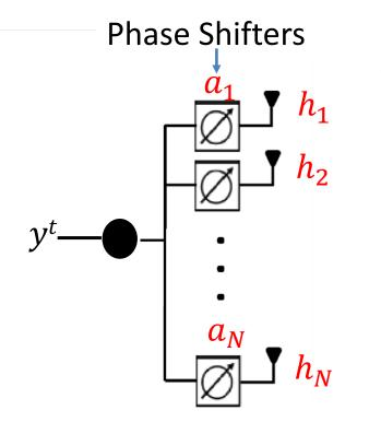
For an Antenna Array:  $\vec{h} = F'\vec{x}$ , F' is Inverse Fourier Matrix  $a_m = e^{j\phi_m}$  $y^{t} = \sum h_{m} e^{j\phi_{m,t}} e^{j2\pi\Delta f_{c}t}$  $= \vec{a}^t \vec{h} = \vec{a}^t F' \vec{x}$
