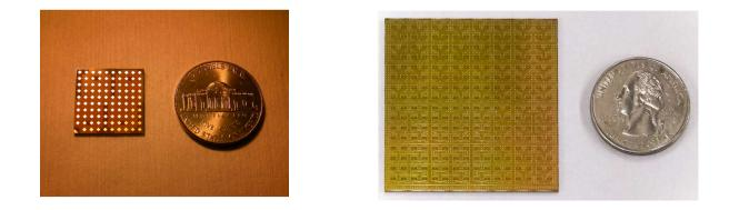
Small Wavelength enables thousands of antennas to be packed into small space
