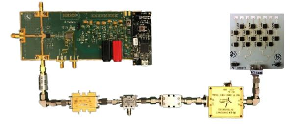
Achieves fast beam alignment: less than 1ms For  $n = 256,100 \times$  faster than 802.11ad and  $10000 \times$  faster than exhaustive search Real-time Applications to Wireless Networks
