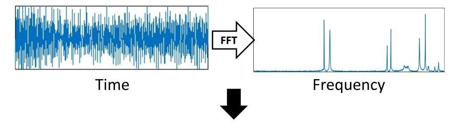
We leverage sparsity to compute the Fourier transform faster than FFT Sparsity appears in GPS, medical imaging, video, audio, astronomy data, seismic data, genomics
