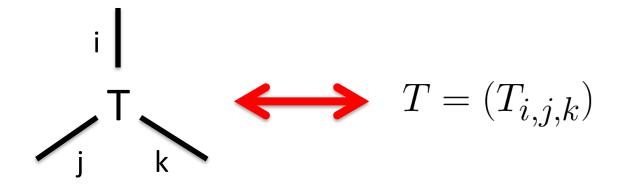
tensors can be attached by summing over connected indices
