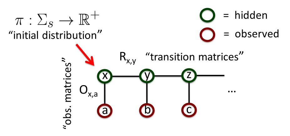
In each sample, we observe a symbol ( $\sum_{O}$ ) at each obs. ( $\bigcirc$ ) node where we sample from  $\pi$  for the start, and propagate it using  $R_{x,y}$ , etc ( $\sum_{S}$ )
